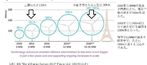
Figure 14.4 Evolution of the largest commercially available wind turbines
